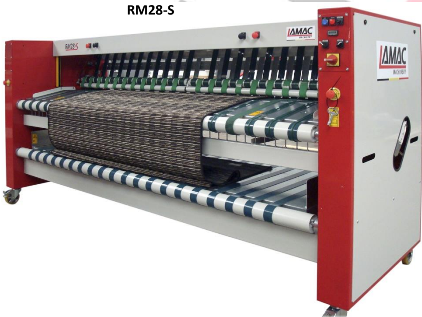
Option: extra feeding belt under machine
